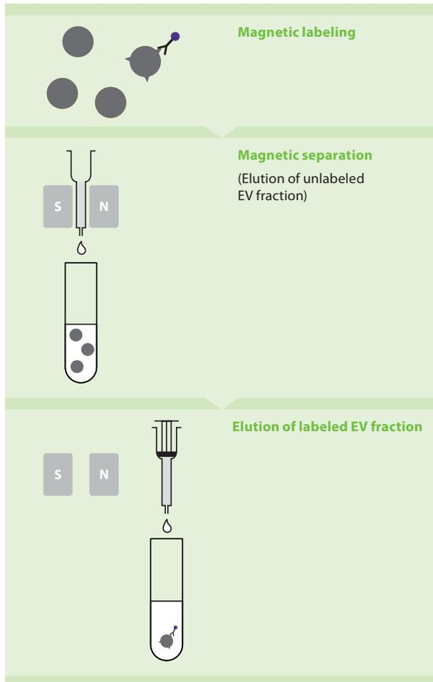
**Figure 1:** Principle of magnetic isolation of EVs using an Exosome Isolation Kit.
