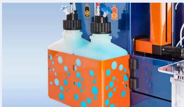
**Figure 6:** Bottle illumination is designed to indicate instrument status.
