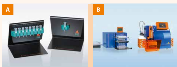
Figure 5: Fast manual separation with the (A) OctoMACS Separator and MS columns on the MACS MultiStand or automated cell separation with the (B) MultiMACS Cell24 Separator Plus and the autoMACS Pro Separator.
